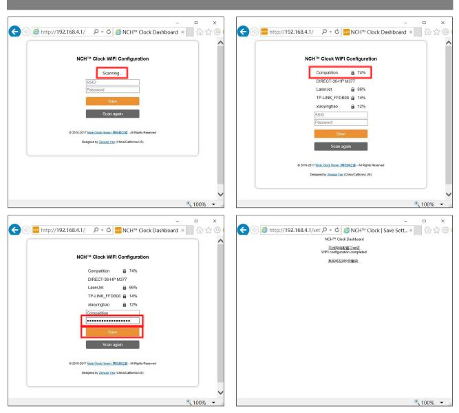
After the WIFI configuration is completed, The Omnixie Will reboot and connect to the WIFI automatically. If the connection is successful, the WIFI status indicator will light **yellow** or **green**. If WIFI status indicator still red after rebooting, it indicates that the WIFI password just entered is incorrect, please select again to make settings.
