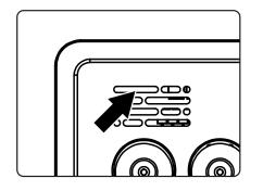
• For the first connection, about 10 seconds after the Omnixie is powered on, the WIFI status indicator will light up in red to indicate that the Omnixie WIFI is not connected to any network and is waiting for configuration. At this point you can use any of the following methods to connect and configure the WIFI network.
